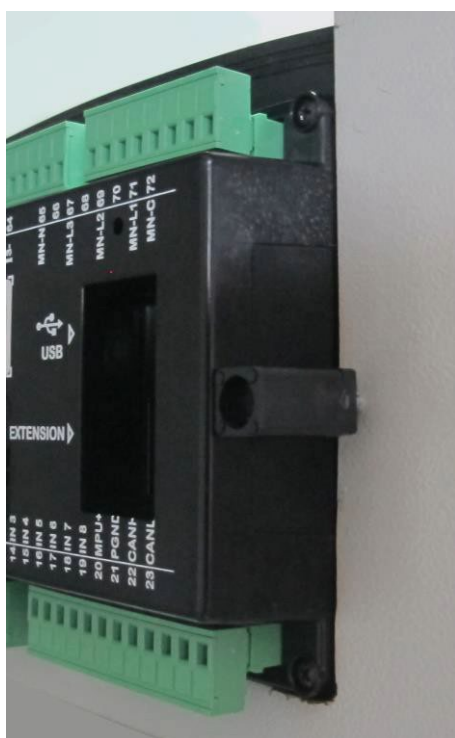
Installation of screw type bracket
