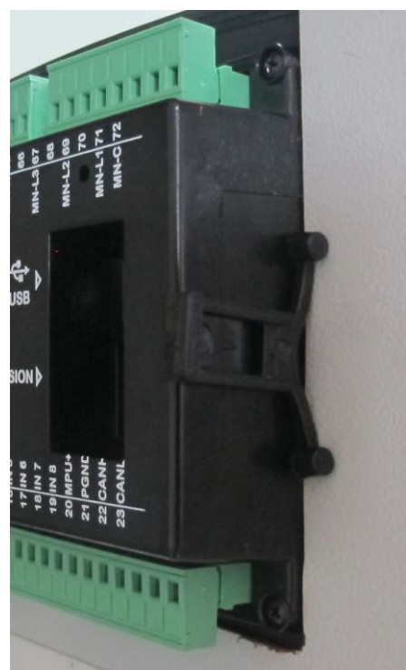
Installation of self retaining type bracket
